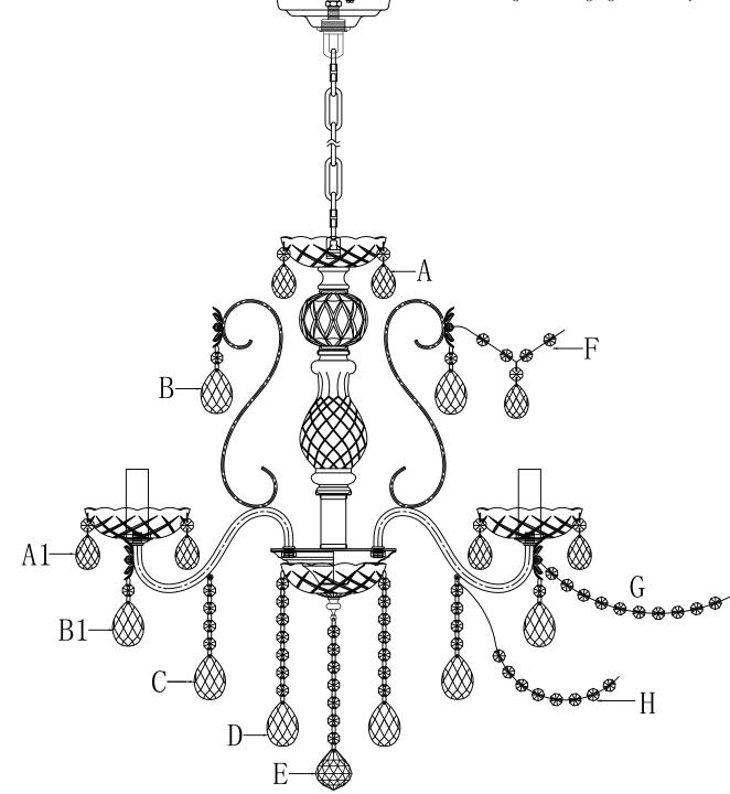
Connect both ends of F with B Connect both ends of H with C
